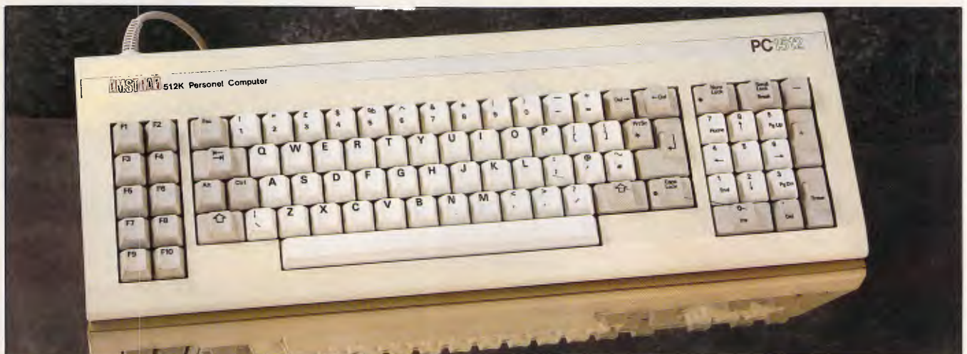
This is not a standard, cheap Amstrad bubble keyboard; the keys are mounted in solid plastic with springs
